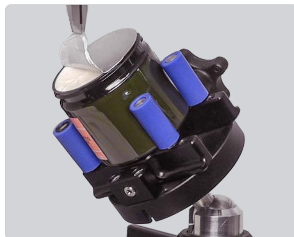
▲ Tamper-evident foil 135° peel
