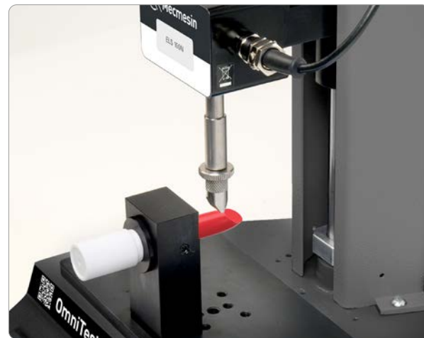
▲ Lipstick bullet break resistance
