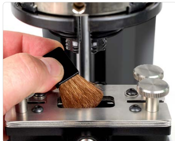
▲ Applicator brush filament pull-out resistance
