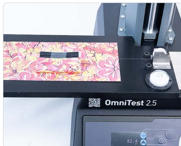
▲ Coefficient of Friction (COF) measurement for packaging print optimisation
