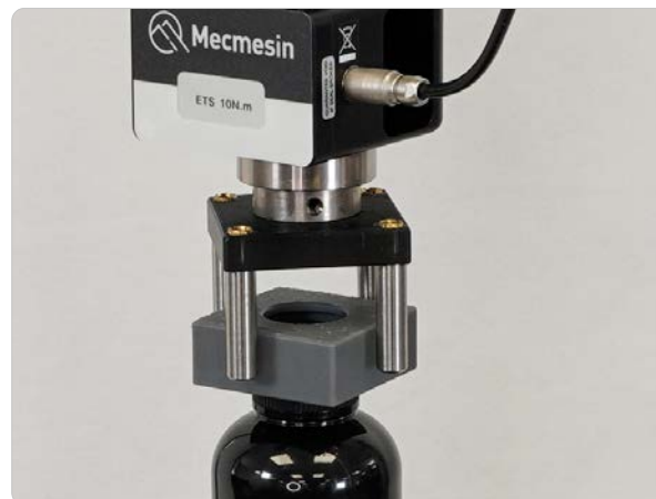
▲ Custom cap mandrel for optimum accuracy
